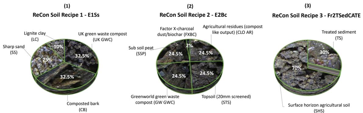
**Figure 1.** ReCon Soil constructed soils and their component materials. 1) ReCon Soil recipe 1 – E1Ss; 2) ReCon Soil recipe 2 – E2Bc; 3) ReCon Soil recipe 3 – Fr2SedCATE.
