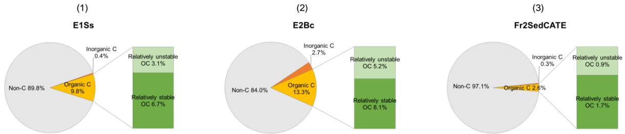
**Figure 3.** Component fractions of three ReCon Soil soil recipes - E1Ss (1); E2Bc (2); and Fr2SedCATE (3): non-carbon (*grey pie slice*), organic carbon (*yellow pie slice*), inorganic carbon (*orange pie slice*); relatively unstable organic carbon (*light green bar*), and relatively stable organic carbon (*dark green bar*).
