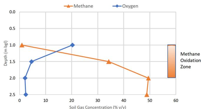
Figure 7: Typical soil gas profile, source zone (WSP).
