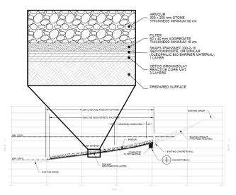
Figure 5: Layering and design of OBB.
