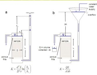
$t = time from h_o to h_i \qquad A = cross sectional area of sample$ Figure 7. Schematic of falling head (a) and constant head (b) permeameter setups
