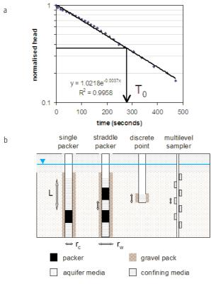
Figure 3. a) example of data from a falling head slug test in unconsolidated porous media. Arrow shows  $T_0$  – the point at which normalised head is 0.37, required in the Hvorslev equation. b) 4 possible slug test configurations.  $r_c$  = casing radius,  $r_w$  = well radius, L = screen length (test interval).
