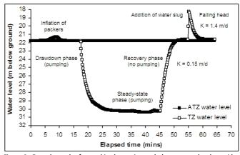
Figure 2. Example results for combined pumping and slug tests undertaken with a straddle-packer arrangement, showing response of water levels within the 2 m test zone (TZ) and above the test zone (ATZ) recorded with pressure transducers during different phases of the test (see text for discussion).
