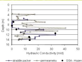
Figure 4. Comparison of K values derived from repacked permeametry and grain size analysis (GSA) of subsampled core, and straddle packer tests performed in a long screened well subsequently installed in the cored hole. Aquifer was an unconsolidated massive layered sand system.
