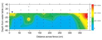
Figure 1. Contour plot of total BTEX concentration ( $\mu$ g/L) across a portion of a plume emanating from a nearby NAPL source underlying a petrol station forecourt. Dots indicate location of multilevel sample ports. Note high concentration gradients. Flow is into the page at ~9 cm/day.
