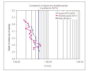
Figure 6. Favourable comparison of dipole and straddle packer derived K values from the Borden Aquifer, Canada. Downward trend of increasing K has been previously noted in that aquifer. Well S07 was installed by direct push without a sand pack.
