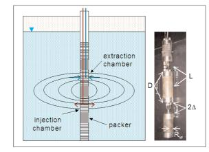
Figure 5. Schematic of dipole assembly in well and resulting idealised flowfield. Design and operational parameters are D (central packer length), L (half dipole length),  $2\Delta$  (chamber length), Q (pump rate). Dipole is constructed to fit a given  $R_{wr}$ , well radius.
