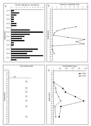
Figure 8. Information used to design installation of MLS to monitor groundwater quality at an unleaded fuel-contaminated site on the Upper Chalk aquifer. Plots show (a) vertical fracture log; (b) aquifer hydraulic conductivity; (c) sample port location; (d) contaminant distribution obtained with completed MLS. Depth (see text) is given metres below forecourt level (mbfl).
