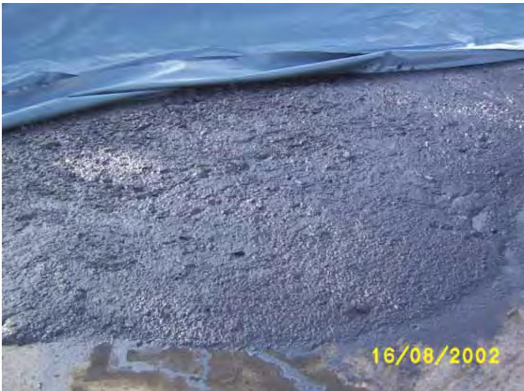
Plate 6.13: Coal tar recovered from the tar tanks for use in the bioreactor trial
