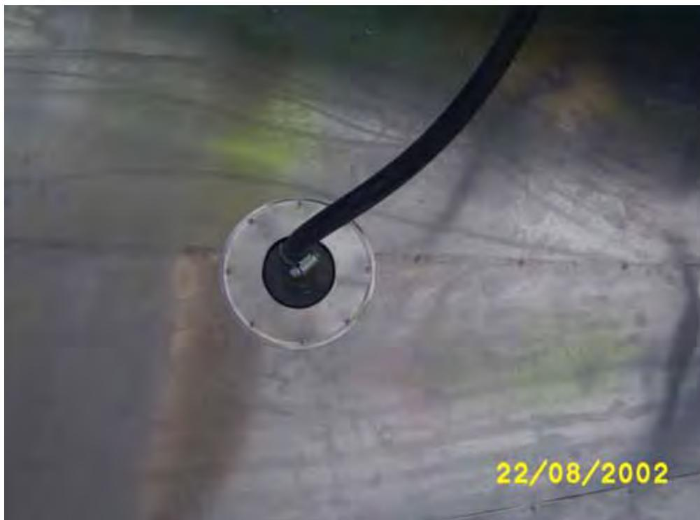
Plate 6.10: Air inlet hose attached to air inlet. Air inlets were positioned around the cone at the base of the bioreactor
