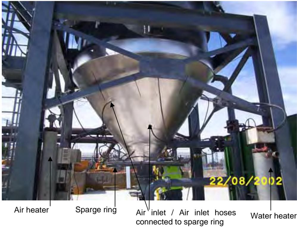
Plate 6.9: Base of bioreactor, construction completed
