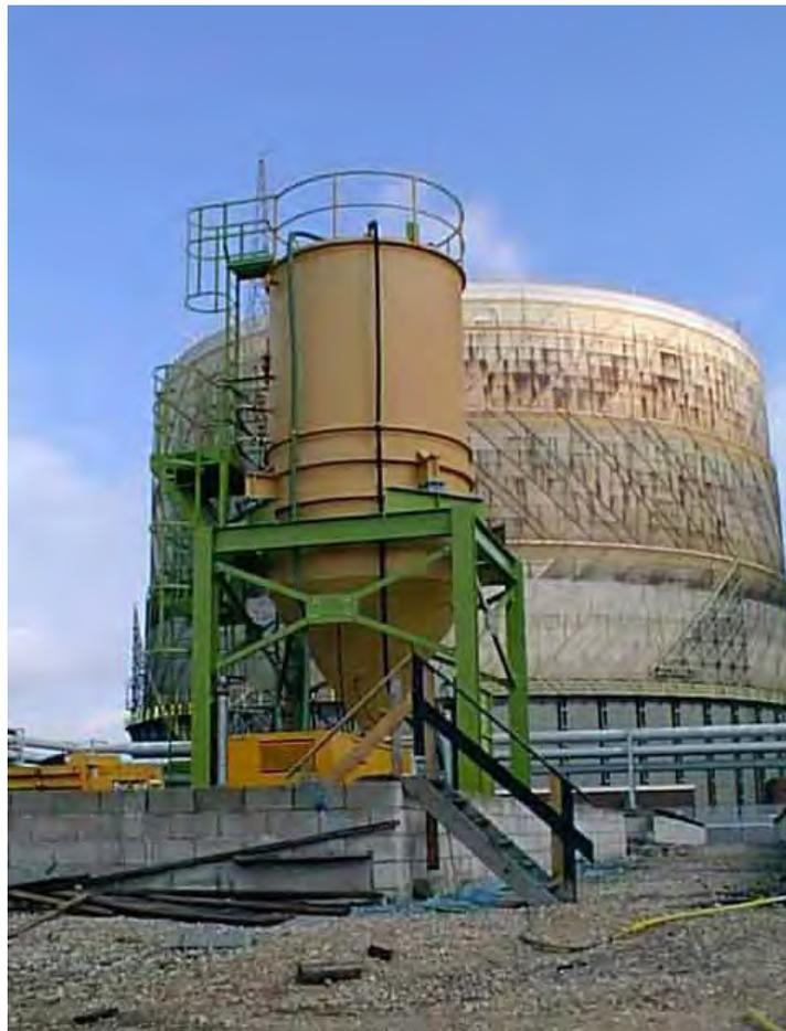
Plate 2.2: The slurry-phase bioreactor after the first trials on a gasworks in northern England
