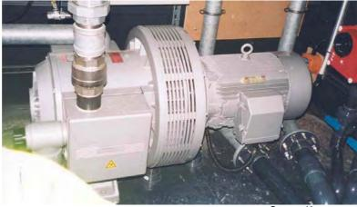
Plate 7.4: Air injection compressor
