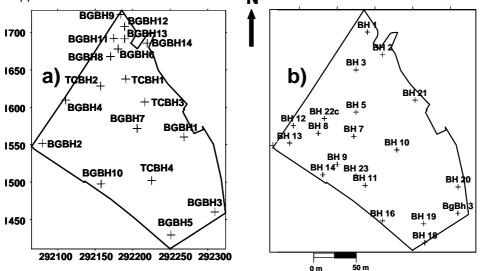
Figure 3.1: Location of boreholes drilled to investigate the extent of groundwater contamination within the site in (a) 2001, and (b) 2003
