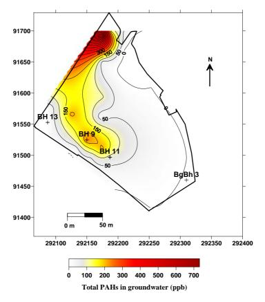
Figure 3.8: Site spatial distribution within groundwater of the EPA 16-PAHs and the position of boreholes in relation to the contaminant plume
