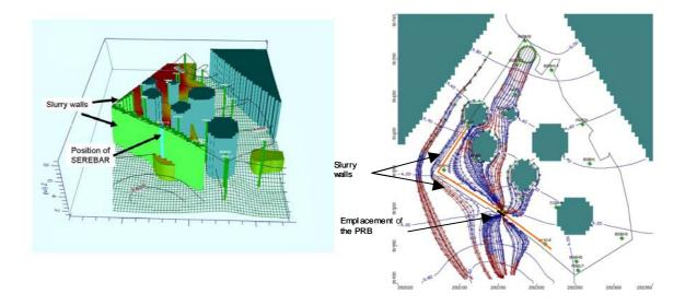
Figure 5.3: Plan of the site showing the position of the slurry walls (the funnel) and the reactive zone (the gate) in 3D (left) and 2D (right). TOC flow delineated as indicator of contamination plume
