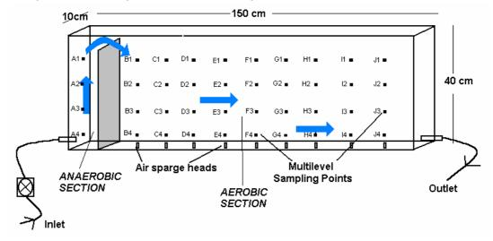
Figure 5.2: Schematic diagram of the bio-barrier
