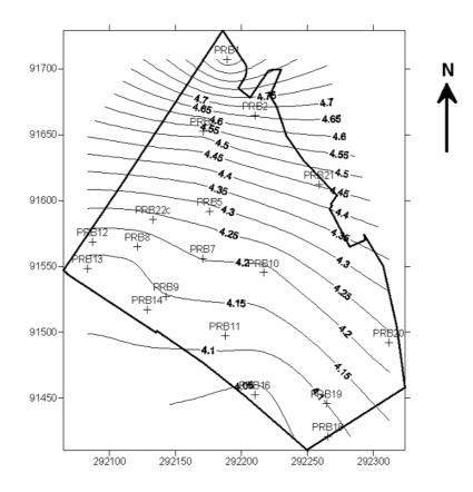
Figure 3.3: Groundwater levels (from monitoring carried out in January 2003)
