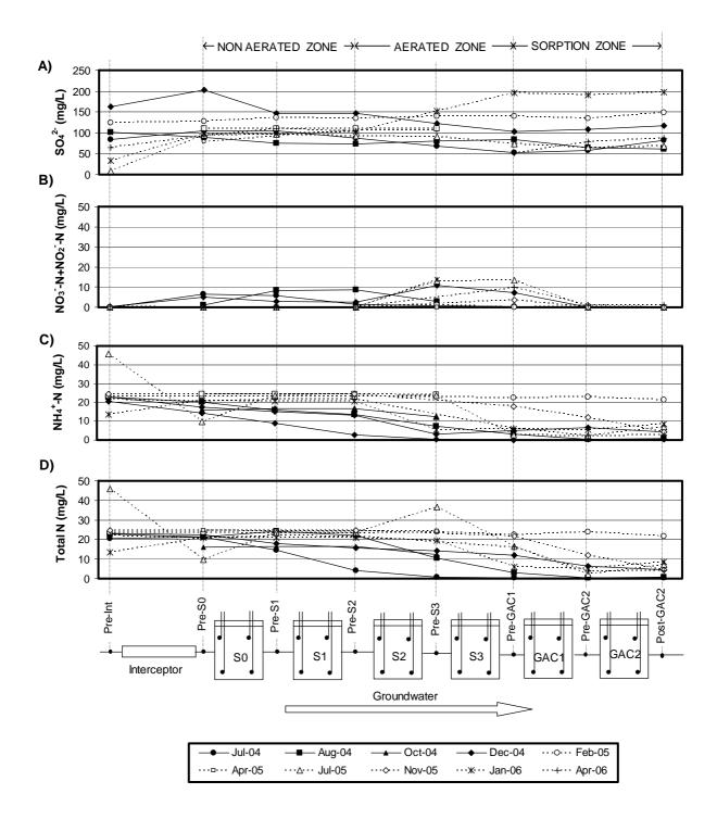
Figure 8.3: Concentration profiles of sulphate and inorganic nitrogen species through the SEREBAR reactors: A) sulphate; B) nitrate+nitrite; C) ammonium; and D) total N, across the barrier for each sampling event. Solid lines indicate concentrations with the original interceptor operating at the design flow rates (before Jan-05) and dashed lines indicate concentrations with the fully sealed interceptor operating at higher flow rates (Gibert *et al.*, 2007)
