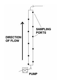
Plate 5.1: Experimental set-up for the treatability column experiments
