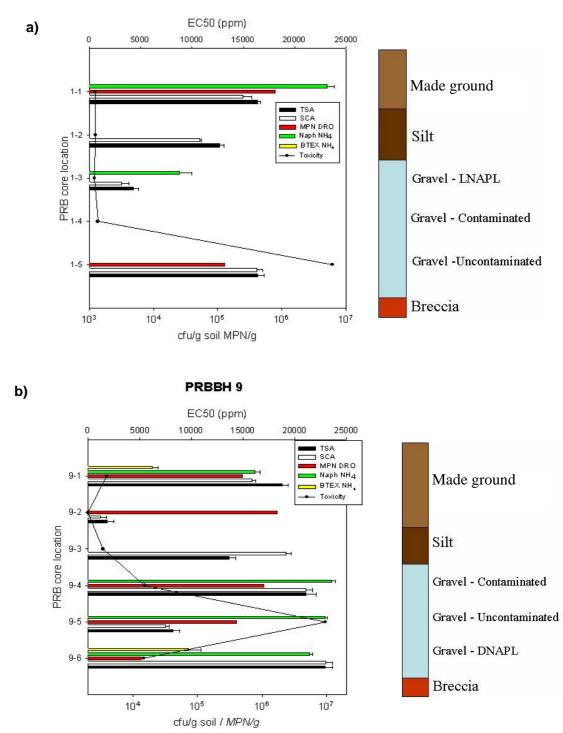
Figure 3.7: Soil core samples total viable heterotrophic counts, bacterial counts on minimal media containing naphthalene or BTEX as the sole source of carbon, and MPN counts on DRO against toxicity for a) BH 1, and b) BH 9. The PRB core location (Y-axis) signifies the sample identity within the named boreholes at various lithologies
