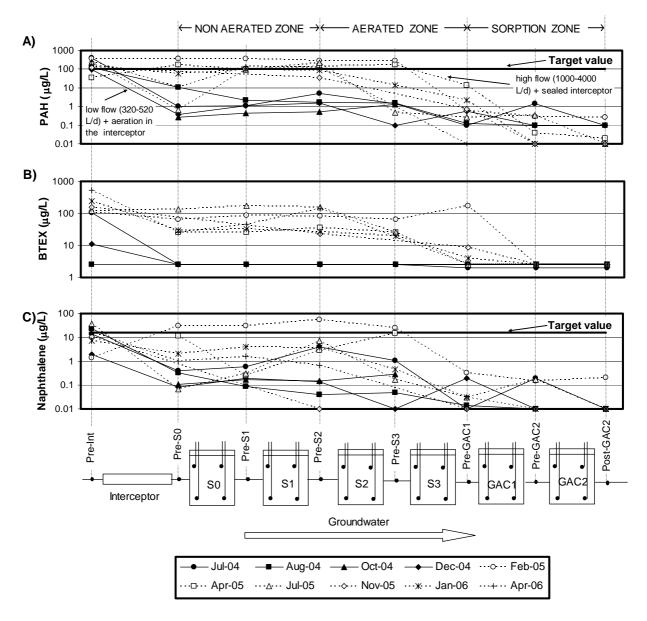
Figure 8.1: Concentration profiles of contaminants of concern through the SEREBAR reactors: A) EPA 16-PAHs; B) BTEX; and C) naphthalene across the barrier for each sampling event. Solid lines indicate concentrations with the original interceptor operating at the design flow rates (before Jan-05) and dashed lines indicate concentrations with the fully sealed interceptor operating at higher flow rates (Gibert *et al.*, 2007)
