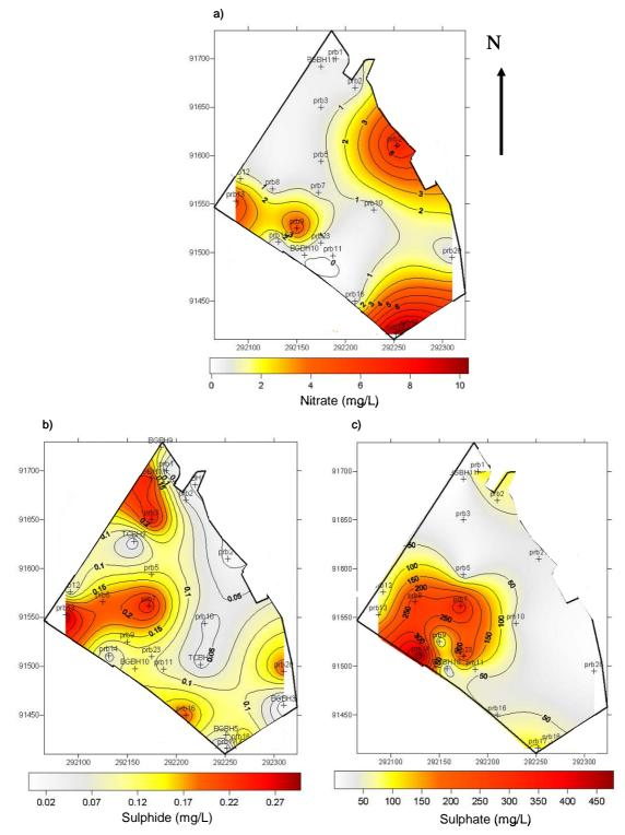
Figure 3.6: Site spatial distribution within groundwater of a) nitrate, b) sulphide and c) sulphate
