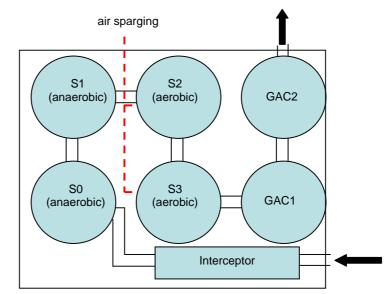
Figure 5.4: Conceptual design of the reactive cells in the SEREBAR
