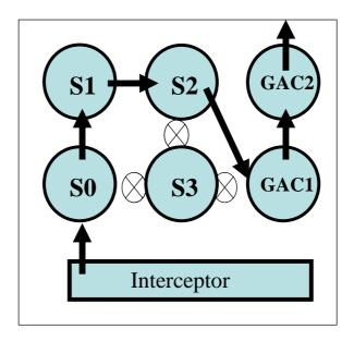
Figure 6.1: Conceptual design of the SEREBAR showing the redirection of groundwater flow following isolation of canister S3
