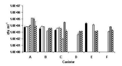
Figure 8.2: Total viable heterotrophic counts of bacteria using naphthalene as the sole carbon source across the SEREBAR reactor after  $2^{1}$ ,  $3^{1}$ ,  $5^{1}$ ,  $6^{1}$ ,  $9^{1}$ ,  $11^{1}$ , and  $14^{1}$  months of operation. Groundwater flow rate was increased from 520 L/d to 4000 L/d after 7 months (Ferguson *et al.*, 2007). The counts are the mean of triplicates with standard errors indicated
