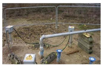
Pilot trial heater wells, extraction well and temperature monitoring wells
