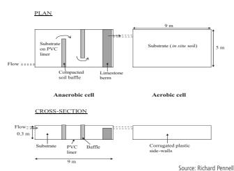
Figure 3: Layout of Gavinswelly pilot-scale constructed wetland in plan and cross-section.
