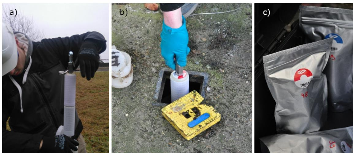
**Figure 3: iFLUX application in the field** a) iFLUX sampler with 2 cartridges, b) VOC cartridge on sampler that slides in monitoring well, c) iFLUX cartridges in their packaging bags.
