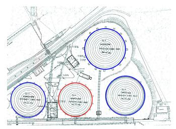
Figure 2: Extract from 1936 site layout plan showing the location of the four gas holders on site. Gas Holder No. 3 is the middle of the four gas holders shown and circled red. Gas Holders Nos 2, 4 and 5 are circled blue. Courtesy of National Gas Archive.
