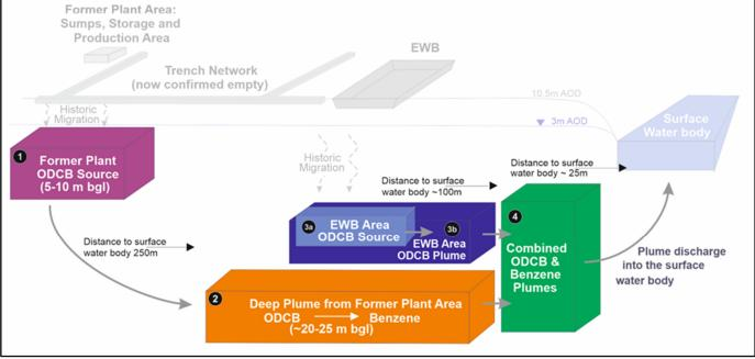
Figure 2: Conceptual site model showing target treatment zones.
