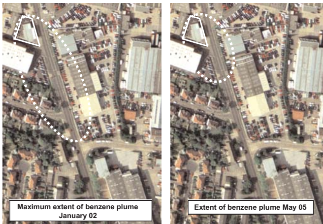
Figure 6: Extent of benzene plume in January 2002 and May 2005 illustrating that the plume has shrunk with time.
