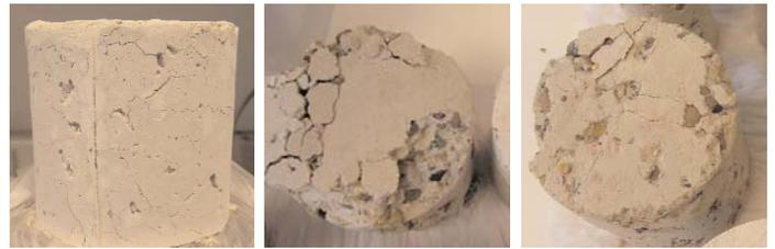
Figure 8. Damage on stabilised/solidified soil samples following different imposed climate scenarios.
