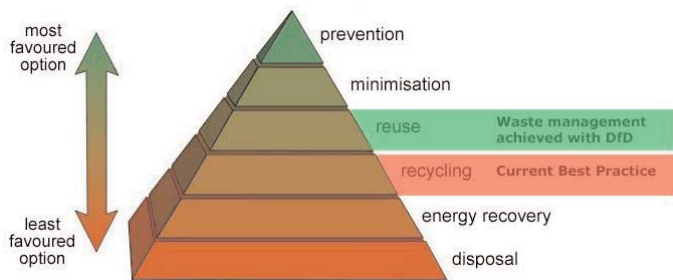
Fig 5. Waste hierarchy indicating current best practice and what can be achieved with DfD.
