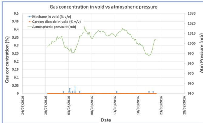
Figure 8. Gas concentrations and atmospheric pressure
