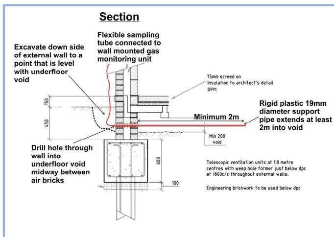
Figure 3. Monitoring point construction.
