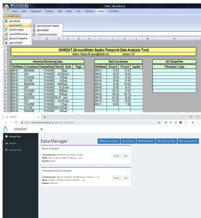
Figure 1. GWSDAT input sheet (top) and on-line GWSDAT data manager (lower) where template can be downloaded and uploaded.
