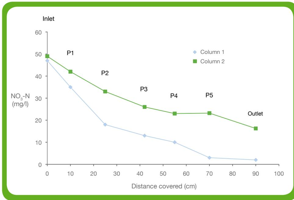
Figure 3.3: Results from the column experiments. Profile of nitrate concentrations (expressed as NO<sub>3</sub><sup>-</sup>-N) along Columns 1 and 2. Different flow rates which equated to average residence times of 6.5 and 1.6 days for Column 1 and 2, respectively.
