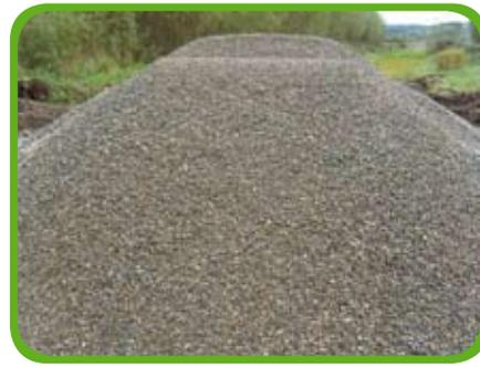
Figure 3.4: Mulch (left) and 5-10 mm gravel (right) used in the NITRABAR
