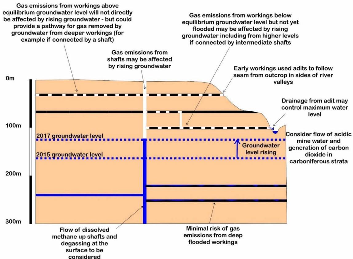
Figure 11.1: Example groundwater conditions and influence on mine gas risk - generalised schematic of Midlothian Coal Field (based on groundwater conditions in Todd *et al.*, 2019). For a larger version, see page 71.
