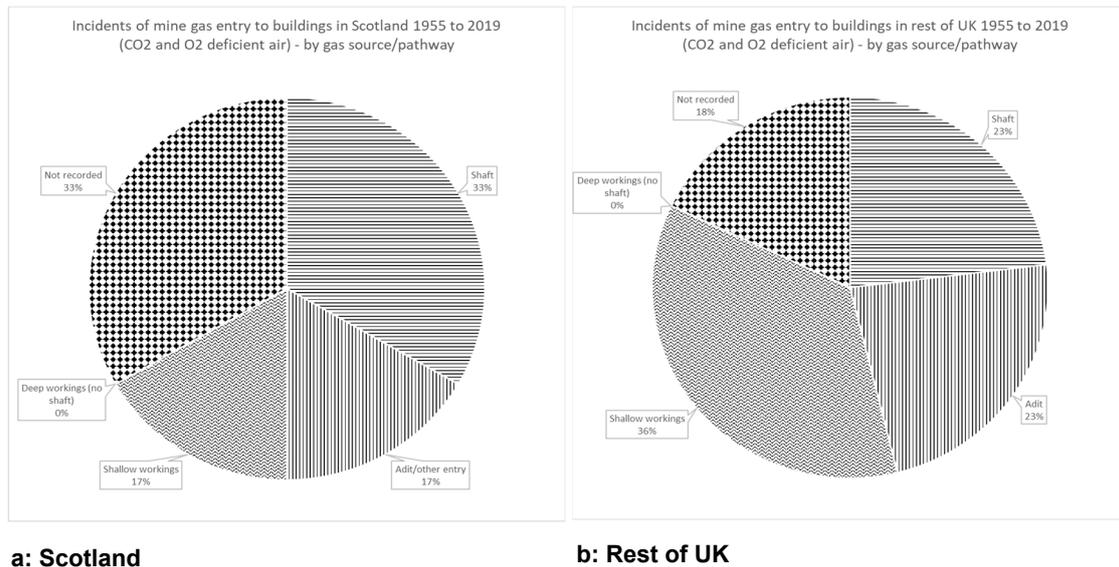
**Figure 5.1: Incidents of carbon dioxide entry to buildings from mine workings (a) Scotland (b) rest of UK (percentages refer to the proportion of the total incidents that were related to the source/pathway).** For a larger version, see page 67.
