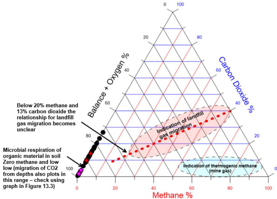
**Figure 13.2: Ternary plot showing aerobic soil respiration, thermogenic methane and landfill gas migration zone (after Wilson *et al.*, 2018b).** For a larger version, see page 74.
