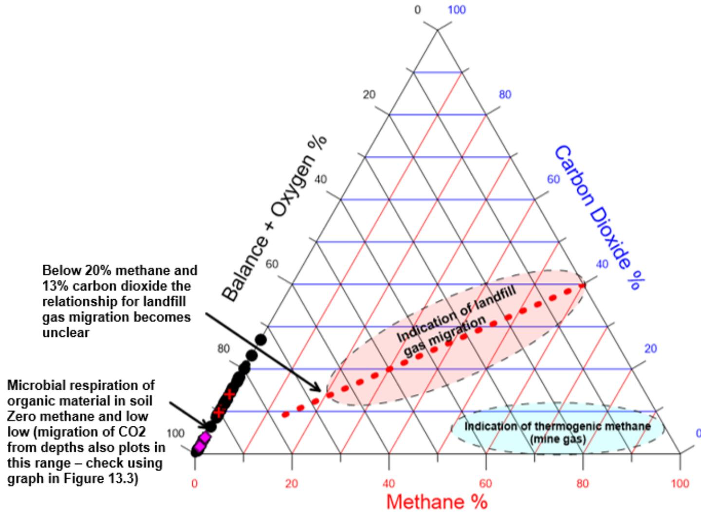
Figure 13.2: Ternary plot showing aerobic soil respiration, thermogenic methane and landfill gas migration zone (after Wilson et al., 2018) – page 39.
