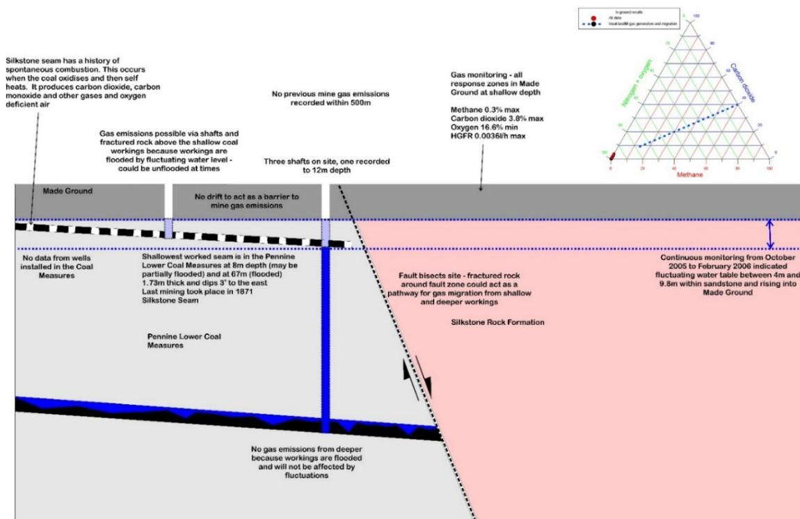
Figure A4.3: CSM for a site with shallow mine workings and shafts. For a larger version see page 78.
