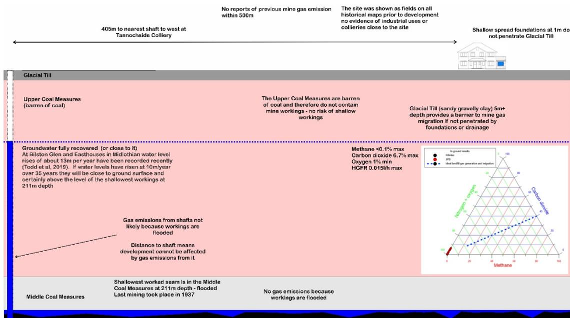
Figure A4.1: CSM for a site with deep flooded workings and no nearby shafts. For a larger version, see page 76.
