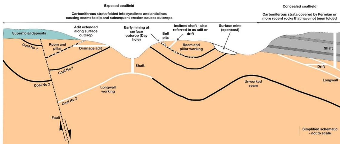
1. Early mining of coal from surface outcrops. Also occurred during 1920s/30s in some areas (e.g. from cellars in northeast England). Small scale or with short adits driven into slopes or hillsides where coal outcropped (short due to lack of ventilation and roof support). These workings were not recorded. The further from the outcrop and deeper the seam, the less likely they are to be present.
