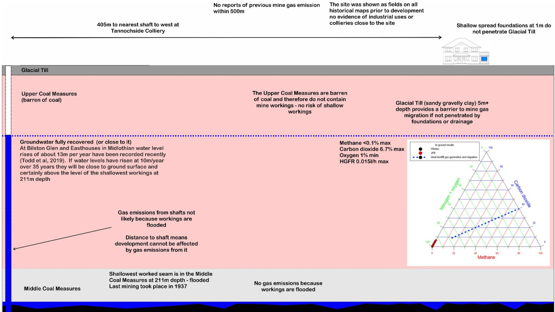
Figure A4.1: CSM for a site with deep flooded workings and no nearby shafts – page 61.
