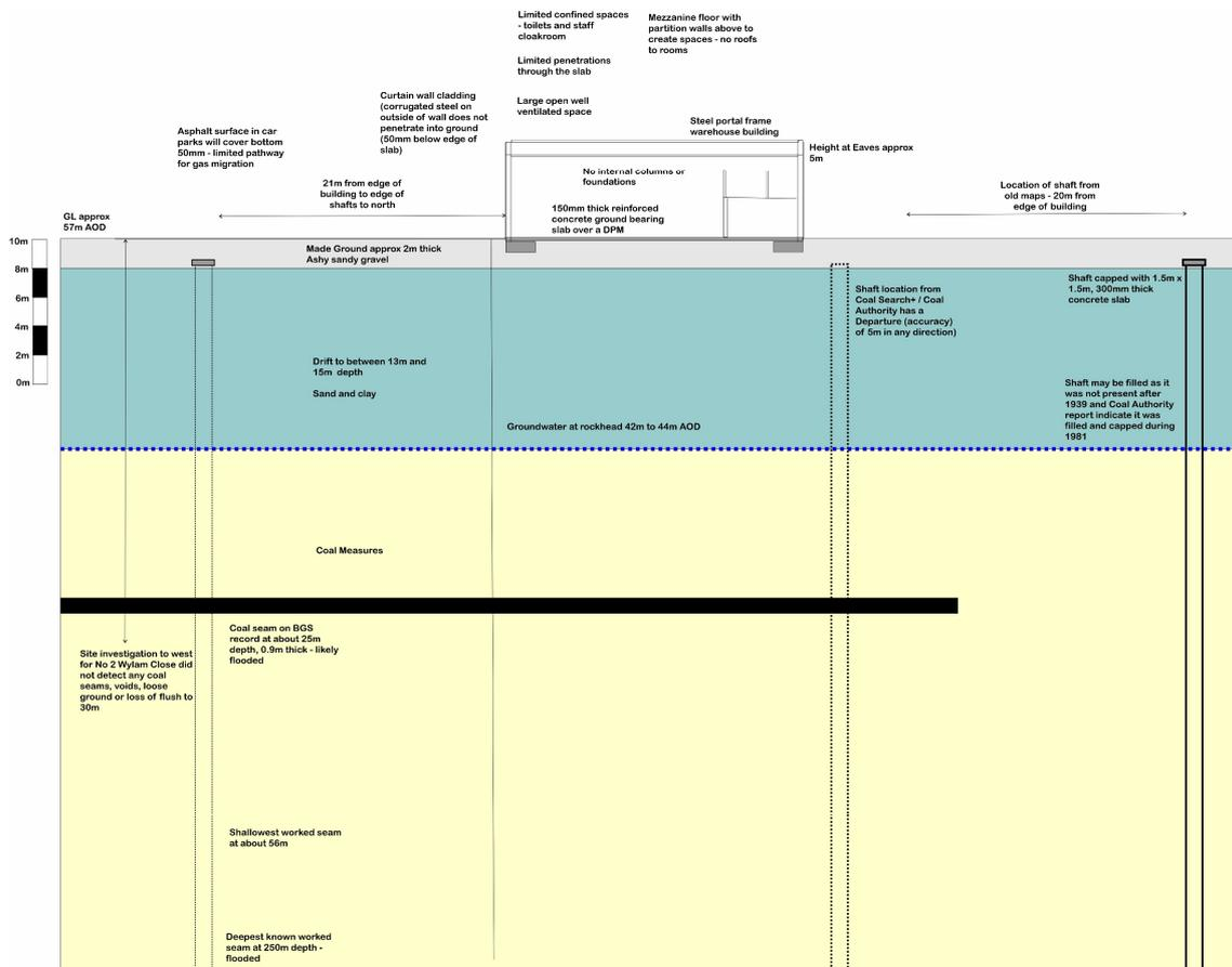
Figure A4.2: CSM for existing building within former colliery. For a larger version, see page 77.
