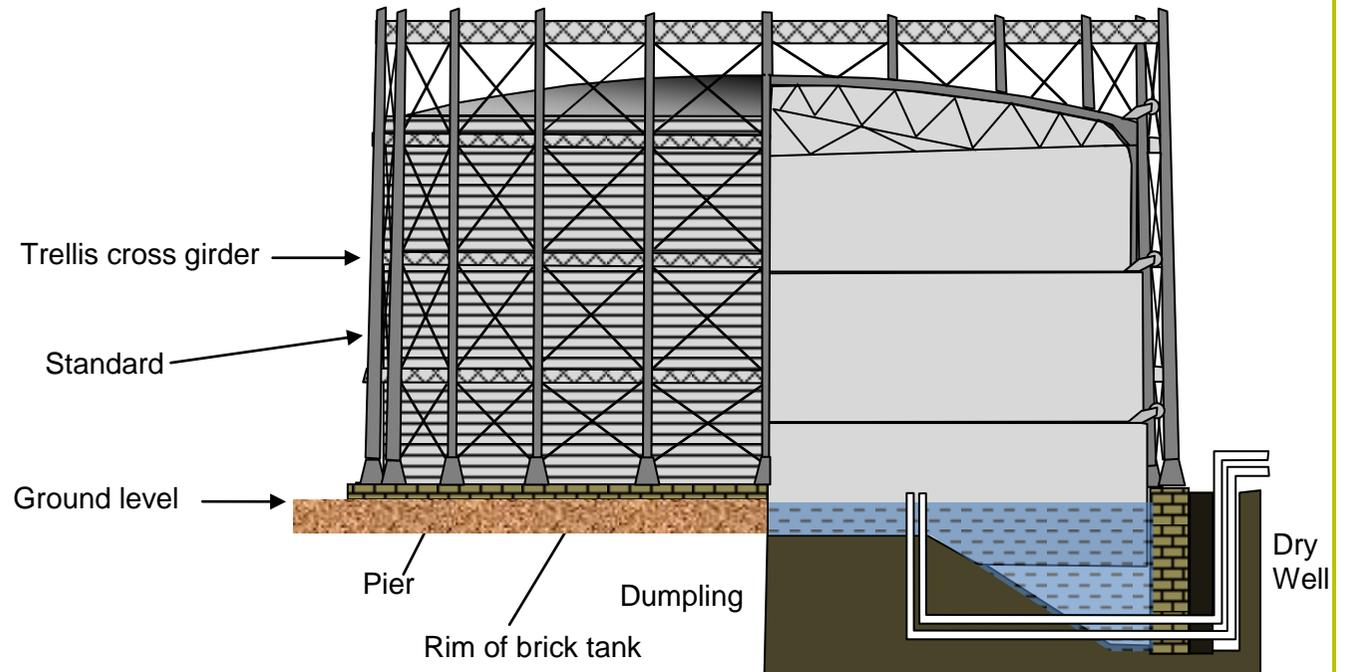
**Figure 4. A schematic diagram of a guide-framed gasholder with a below-ground tank. Source: Russell Thomas.**
