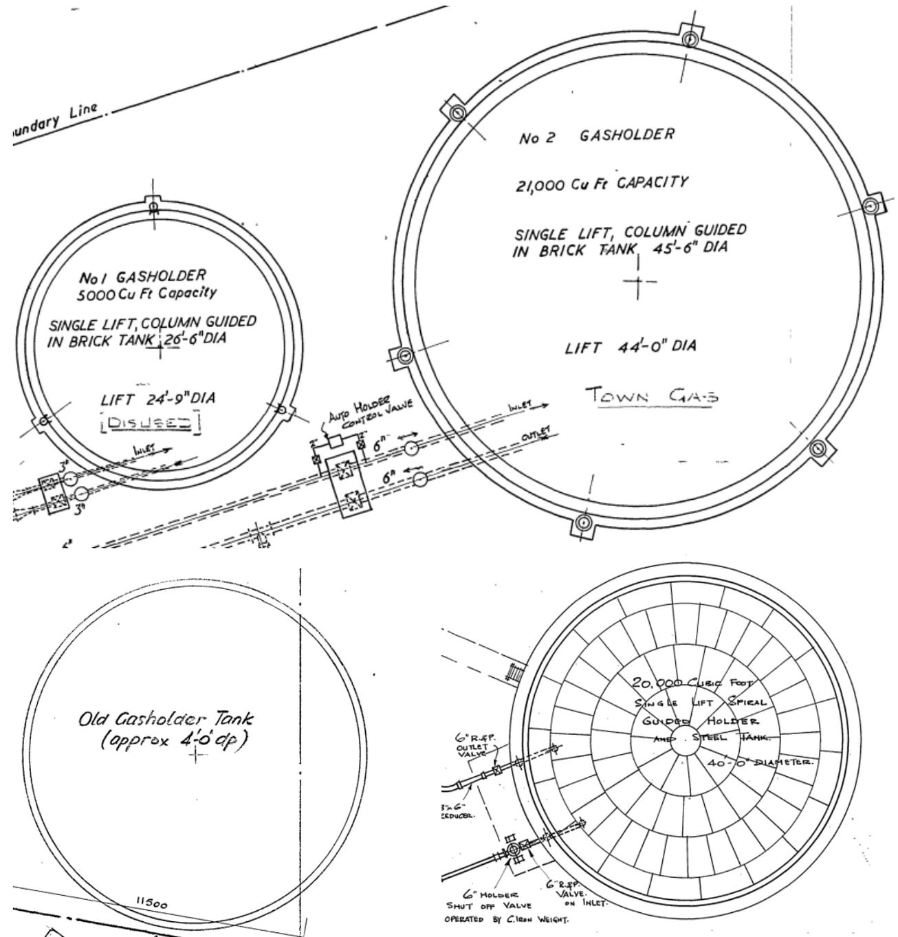
Figure 15. Examples of details of gasholders tanks found on gasholder plans.
