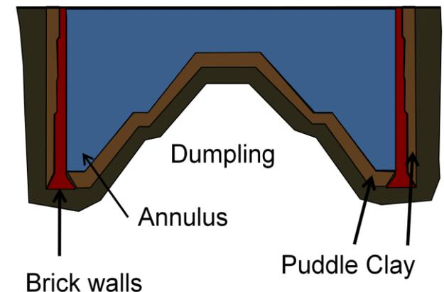
**Figure 12. Schematic of a gasholder tank with a dumpling and annulus. Source: Russell Thomas.**
