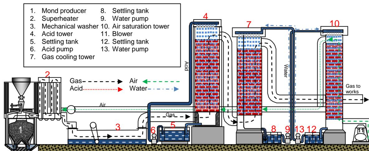
**Figure 5. The Mond system of gas production and ammonia recovery. Based on historical process drawings. Source: Russell Thomas.**
