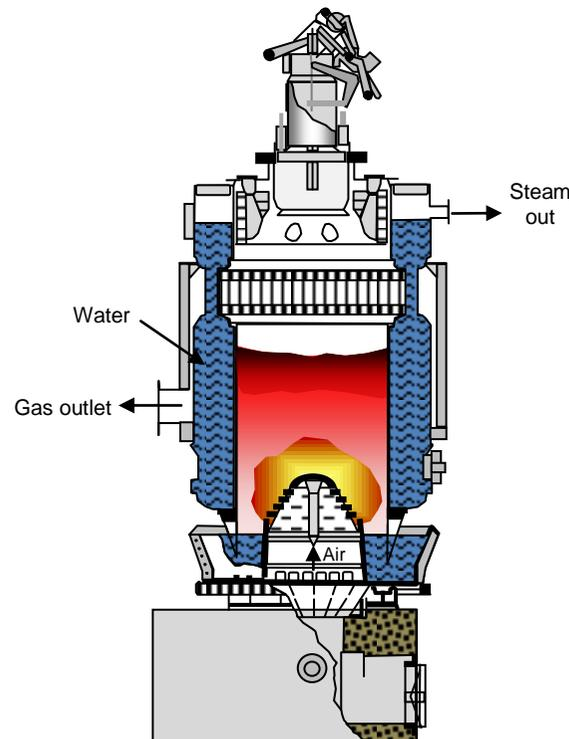
**Figure 7. Cross section of a Marishka type gas producer. Based on a historical drawing, Source: Russell Thomas.**
