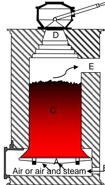
**Figure 2. Gas producer working with air or air and steam.** Source: Russell Thomas.
