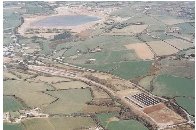
Figure 1: Aerial view of the Wheal Jane Mine complex. Left background shows tailings pond. The pilot passive treatment plant (PPTP) is shown occupying the Carnon River valley in the foreground left to right.
