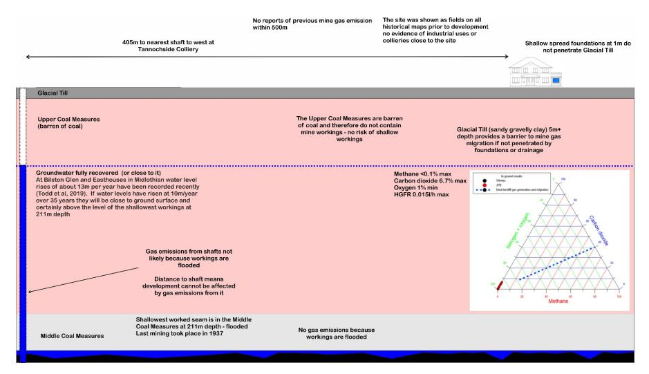
Figure A4.1: CSM for a site with deep flooded workings and no nearby shafts - page 61.
