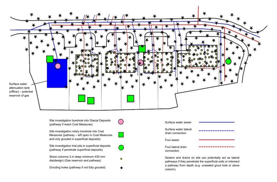
Figure 10.2: Complexity of pathways and gas reservoirs introduced by the development construction – page 20.
