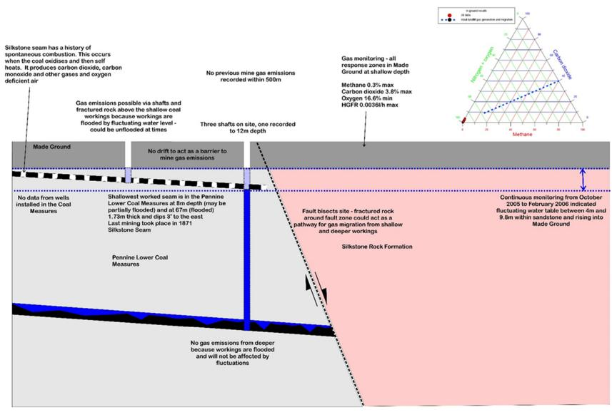
Figure A4.3: CSM for a site with shallow mine workings and shafts - page 64.
