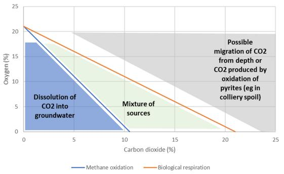
Figure 13.3: Stoichiometric assessment of carbon dioxide and oxygen. For a larger version, see page 75
