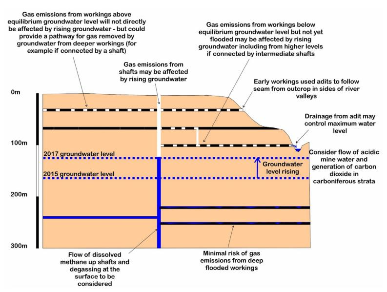
Figure 11.1: Example groundwater conditions and influence on mine gas risk (based on groundwater conditions in Todd et al., 2019) – page 24.
