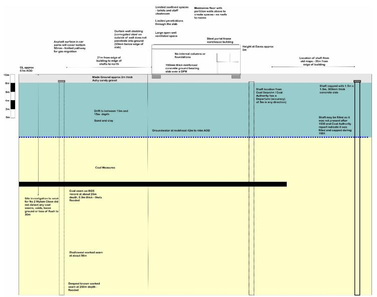
Figure A4.2: CSM for existing building within former colliery – page 62.
