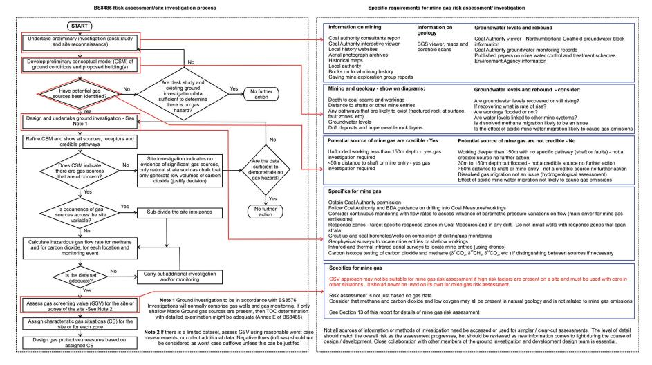
Figure 12.1: Flow chart for gas risk assessment with specific considerations for mine gas assessment. The left hand side has been adapted from BS 8485 and the right hand side shows how the specific considerations for mine gas assessment described in this document follow the generic flow chart from BS 8485 – page 27.
