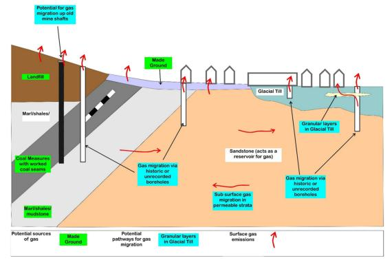
Figure A4.4: CSM for a site with old site investigation boreholes. For a larger version, see page 79.
