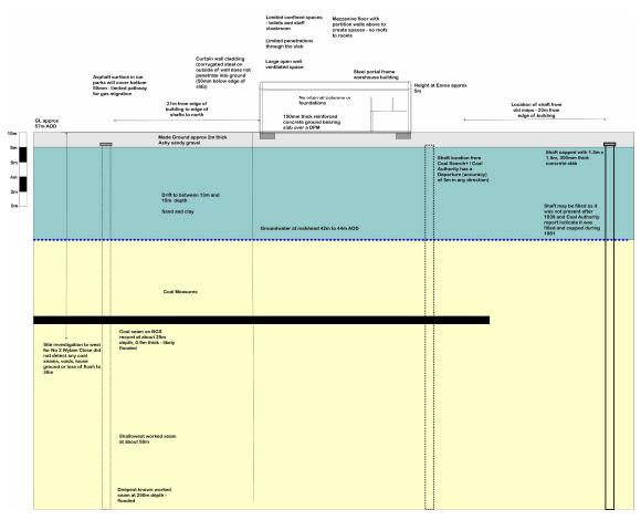
Figure A4.2: CSM for existing building within former colliery. For a larger version, see page 77.
