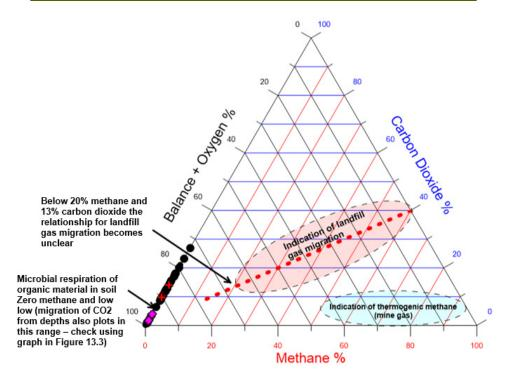
Figure 13.2: Ternary plot showing aerobic soil respiration, thermogenic methane and landfill gas migration zone (after Wilson et al., 2018b). For a larger version, see page 74.
