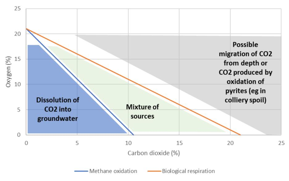
Figure 13.3: Stoichiometric assessment of carbon dioxide and oxygen - page 39.
