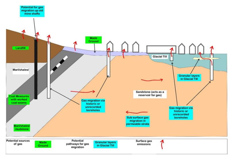
Figure A4.4: CSM for a site with old site investigation boreholes – page 66.
