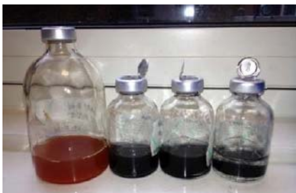
Figure 5. Ferrihydrite (left), large bottle is control without bacteria and the three small bottles are replicates containing Geobacter sulfurreducens , which is reducing ferrihydrite to form bionanomagnetite.
