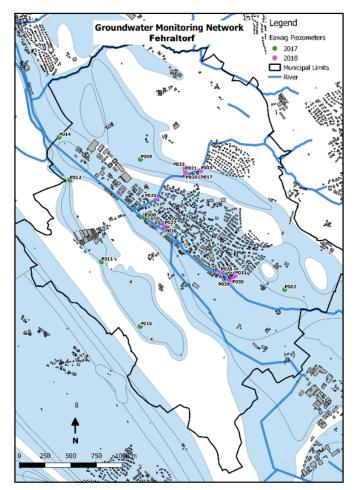
Figure 1: Shallow groundwater monitoring wells installed in Fehraltorf through the course of this study. The main body of the aquifer is shaded in light blue.
