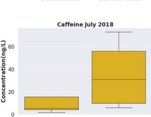
Figure 2: Concentrations of *caffeine* measured in groundwater and surface water in Fehraltorf. *Caffeine* is an indicator for untreated wastewater in the environment.
