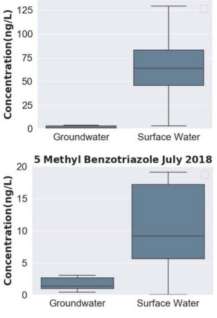
Figure 4: Concentrations of *5-methyl-benzotriazole* measured in Fehraltorf. *Benzotriazole* is mainly thought to be an indicator of industrial activity.
