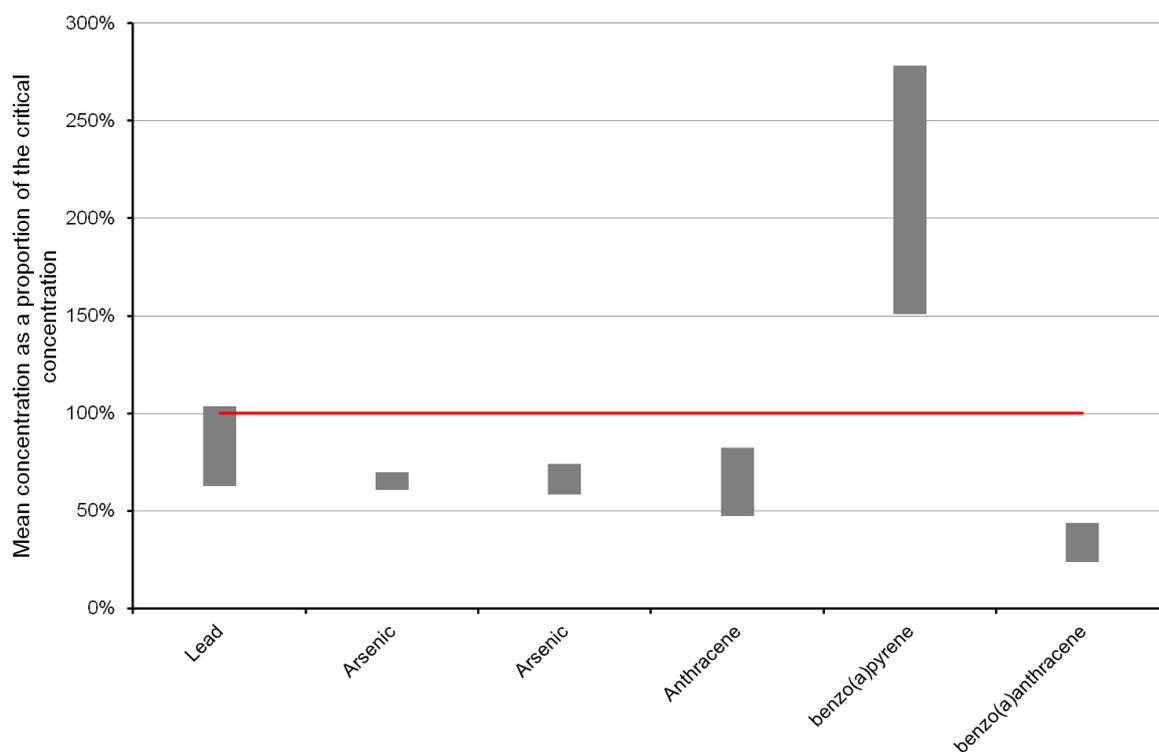
Figure 3: Interval (95% one-tailed) for the mean concentration of contaminant
