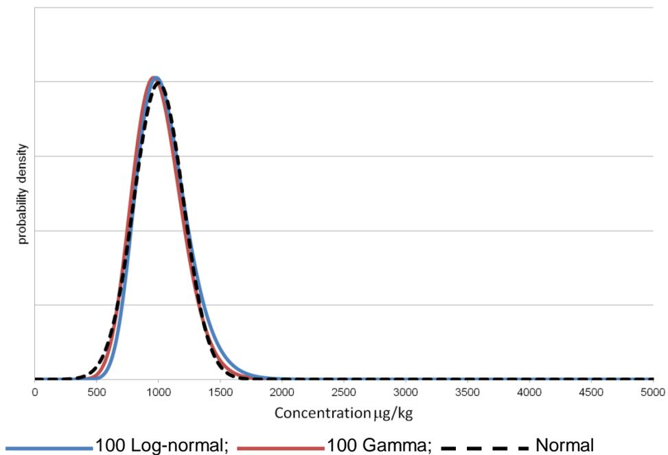
Figure 2: Probability distribution for the mean of 100 samples taken from contaminated land with the same mean and variation but two different distributions.
