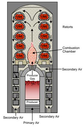
Figure 6. Cross section of a horizontal retort, showing the gas producer. Based on historical drawings, Source: Russell Thomas.
