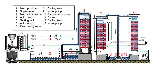
Figure 5. The Mond system of gas production and ammonia recovery. Based on historical process drawings. Source: Russell Thomas.
