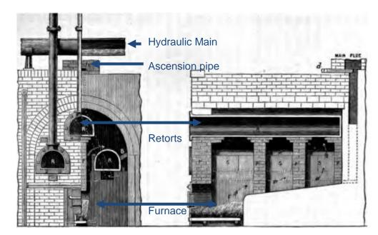
Figure 2. A schematic of a simple bench of three directly fired retorts which would be found in a small gasworks, attributed to Samuel Clegg Jnr. Source: Russell Thomas.
