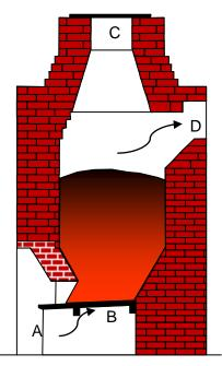
Figure 1. Bischof Gas Producer. Air was drawn into the producer (A) through the fire bars (B) and fuel, exiting via the vent (D). Fuel was loaded via door C. Source: Russell Thomas.
