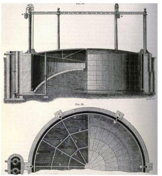
Figure 6. Drawing of an early single-lift gasholder with counterweights and a brick below-ground tank. From 'A Practical Treatise on the Manufacture and Distribution of Coal Gas' by William Richards, 1877.
