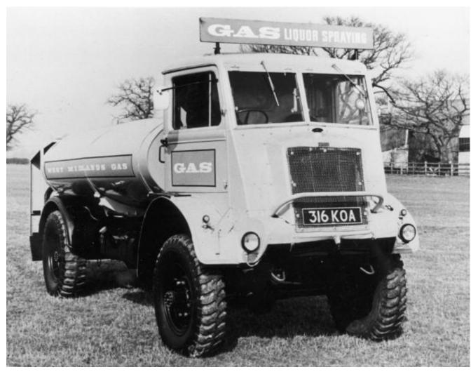
Photograph 60. A tanker used for spraying ammoniacal liquor on agricultural land.
