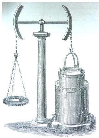
Figure 1. A drawing of the gasholder developed by Antoine Lavoisier, which appeared in his work 'Opuscules physiques et chimiques'. From King's Treatise Vol. II, 1879.
