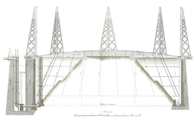
Figure 3. Design of an early gas holder taken from 'A Practical Treatise on the Manufacture and Distribution of Coal Gas' by Samuel Clegg Junior. This simple design shows many of the features common in later gasholders. Note the basic guiding of the gasholder vessel by metal brackets with eyelets running on cylindrical metal bars; these were later replaced by guided rollers.
