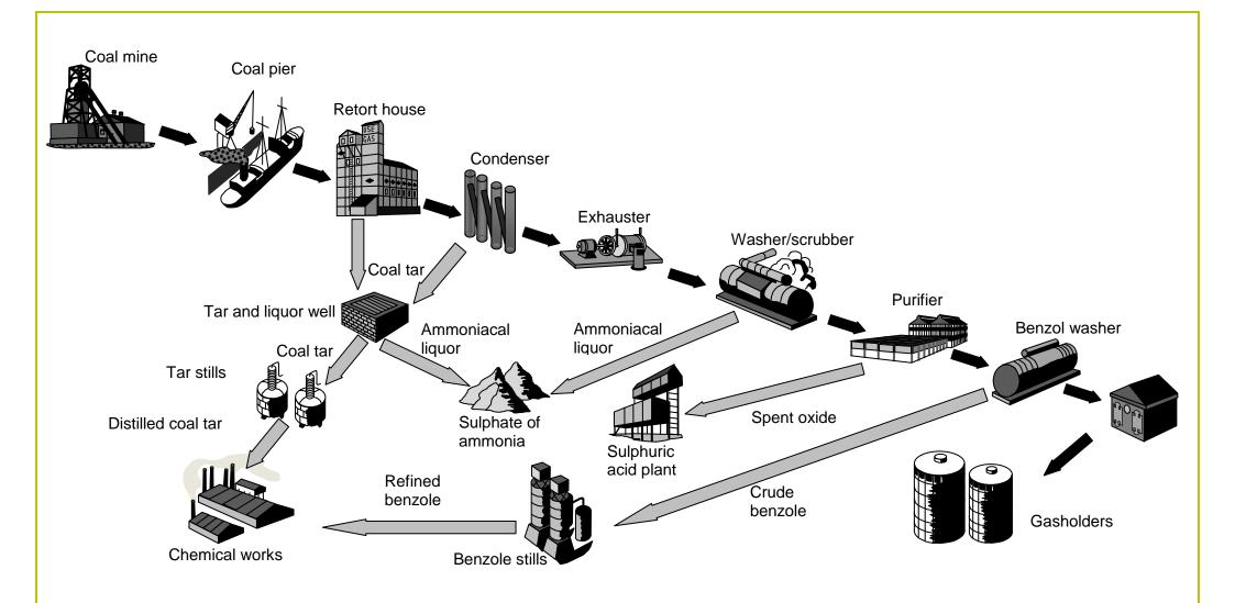
Figure 12. The production of town gas from coal. The black arrows show the progress of the gas through the plant and the grey arrows show the processing of the by-products. Source: Russell Thomas.
