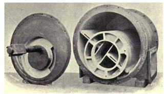
Photograph 28. The internal workings of an exhauster.
