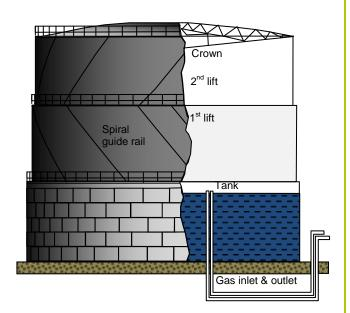
Figure 9. Schematic of a spiral-guided gasholder with an above-ground tank, showing the internal detail and water level. Source: Russell Thomas.
