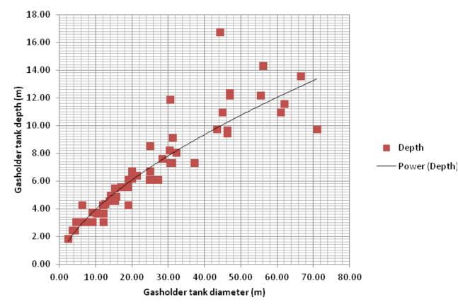
Figure 16. A plot of the gasholder tank diameter against depth for brick, stone, concrete and composite tanks. Source: Russell Thomas.
