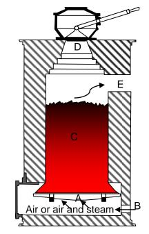
Figure 2. Gas producer working with air or air and steam. Source: Russell Thomas.
