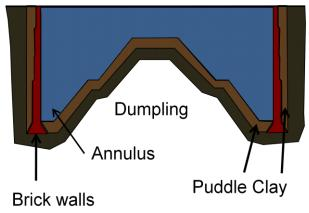
Figure 12. Schematic of a gasholder tank with a dumpling and annulus. Source: Russell Thomas.
