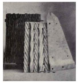
Photograph 33. The corrugated filter material used inside the standard washer-scrubber. Source: *Modern Gasworks Practice*, 1916.
