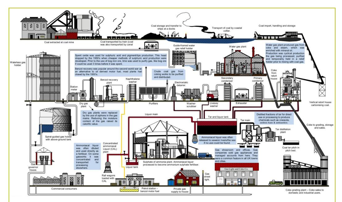
Figure 13. The production of gas from coal and the manufacture of by-products on a large gasworks, showing the process from the mining of the coal to the distribution in the gas mains. Source: Russell Thomas.
