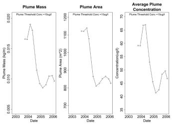
Figure 3. Example of the summary output of plume metrics: plume mass (left), plume area (mid), average concentration (right).
